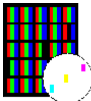
Cluster pixel defect type 3b Sub-pixels/dots in a cluster area constantly dark
