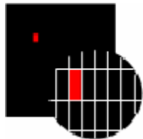
Pixel defect type 3a Sub-pixel/dot (red, blue, green) constantly lit
