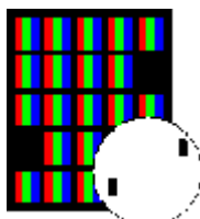
Cluster pixel defect type 2 Pixels in a cluster area constantly dark
