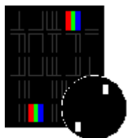
Cluster pixel defect type 1 Pixels in a cluster area constantly lit
