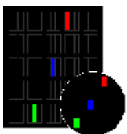
Cluster pixel defect type 3a
