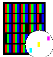
Cluster pixel defect type 3b
