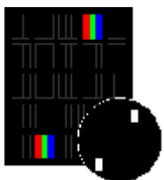
Cluster pixel defect type 1
