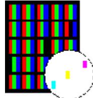
Cluster pixel defect type 3b Sub-pixels/dots in a cluster area constantly
