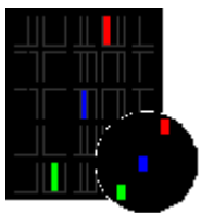
Cluster pixel defect type 3a Sub-pixels/dots in a cluster area constantly lit dark
