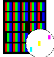
Cluster pixel defect type 3b Sub-pixels/dots in a cluster area constantly dark
